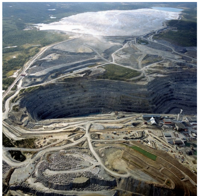
Figure 3 The Aitik copper mine with the open pit, with waste rock dumps in the foreground and the tailings impoundment in the background (photo by Boliden Mineral).
